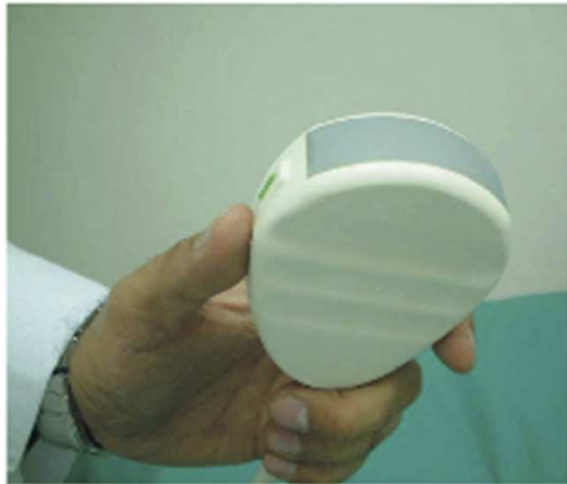
Fig. 6. A curvilinear probe and the format of the scan lines.
