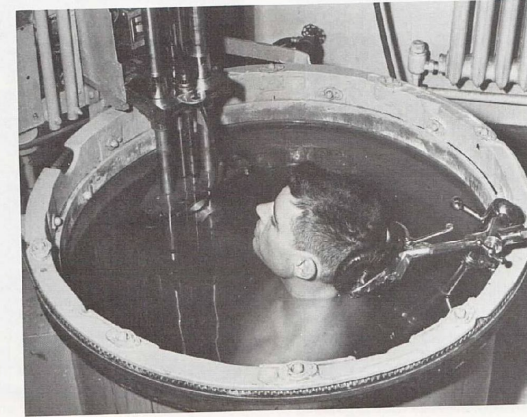
Fig. 1-3. Scanning position for transverse cross-section of the neck. The 2 1/2-inch focused transducer is seen just below the water level. The transducer carriage travels around the tank on the outside track.
